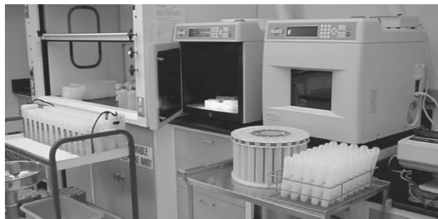
Fig. 1. Professional multimode MW reactor MARS-S (CEM)
